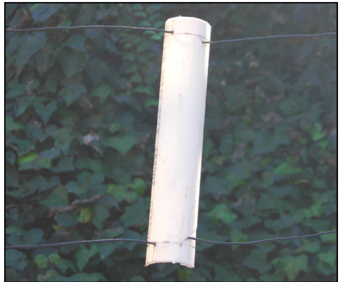
Garden-variety 1-inch PVC is cut into 7-inch long pieces, divided and slotted to accommodate the W3EDP's 84-foot longwire and 17-foot parallel feedline – ingredients for a versatile, lightweight, multi-band, trail-friendly antenna.
