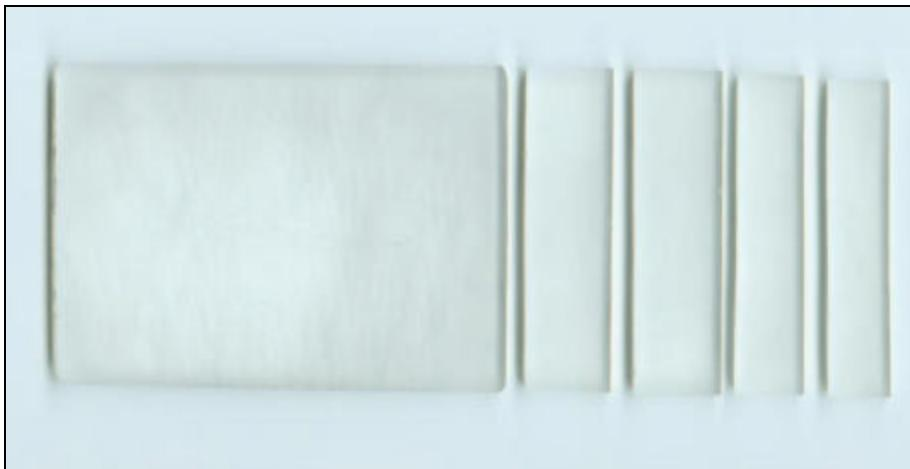
After all the pieces were cut. I sanded all sides and edges to remove any burrs as well as rounding those sharp corners. It will also add a nice opaque look (I hope) to the finished key.
