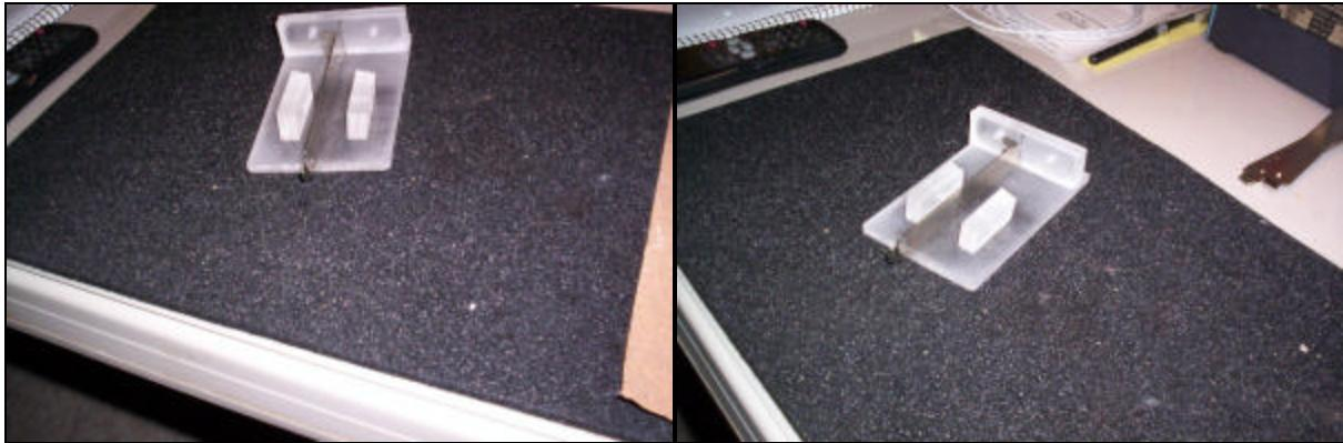
Here I've laid the arm in place to get an idea as to looks. After all of that I drilled from the bottom side some peggin' holes into which I epoxied in two 1/2" long 2-56 screws to reinforce the adjust screw plates. Most likely over kill but did it any way. You'll have to look close to see them.
