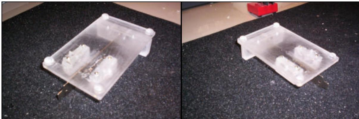
Here is the set up I used on the Adjustment Plates. The inside nut is epoxied on the Adjusting Plate. There 2 nuts and flat washers (6-32) to clamp the wires going to the Back Plate.
