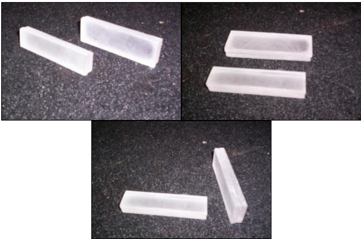
The two pieces for the Back Plate along with the two pieces for the Adjustment Screw Plates have been epoxied together making them 1" X 3.5" X 1/2 and 3/4" X3.5" X 1/2" respectively.
