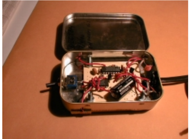
This view shows the board installed into an Altoids tin. The red wires on the left side (top/bottom) attach to scrap pieces of PCB to act as the paddles.
