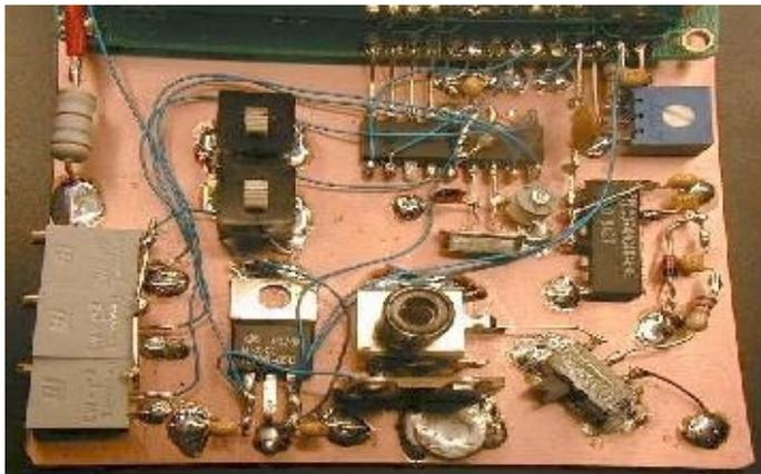
Note the small PIC chip just under the LCD. That's the chip that I demolished by ripping pin 4 clear off the substrate. Bummer just doesn't explain how I felt, but one email to Neil at ADDE made me one happy camper. I told Neil how I destroyed his chip through my own negligence and blundering, Neil said it was no problem and in the interest of customer service he sent me a replacement PIC at NO CHARGE. He did say the next one would be \$20.00 though.
