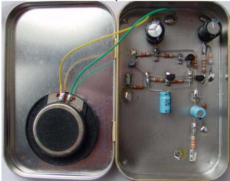
Audio Amp from new ARRL Experimental Methods in RF Design book
