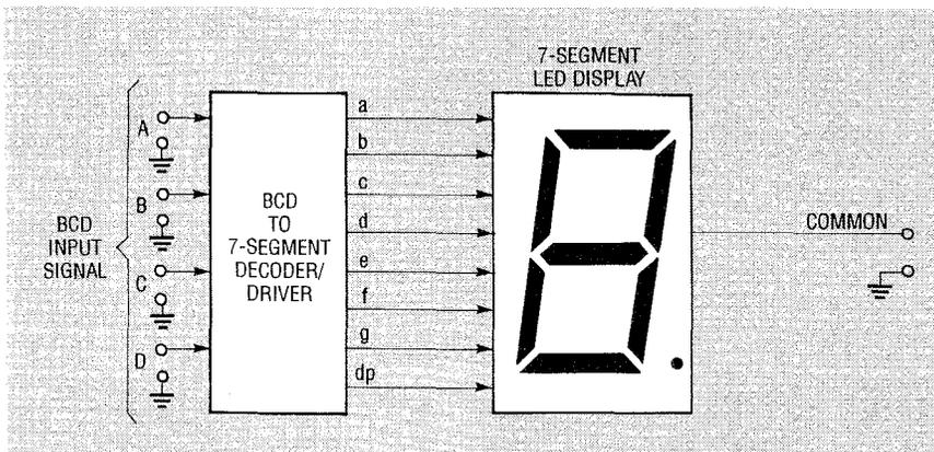
FIG. 21—BASIC CONNECTIONS for a BCD-to-7-segment LED-display decoder/driver.
