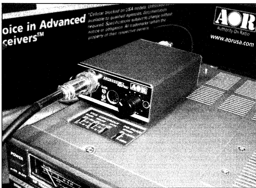
The ARD9000 MK2 Digital Voice Modem from AOR uses the AMBE vocoder and FEC, allowing any SSB radio to operate robust digital voice, while occupying no more bandwidth than an analog SSB signal.
