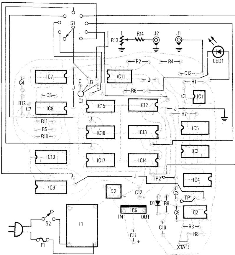
**FIG. 2—TAKE EXTRA CARE THAT VARACTOR DIODE D1 is installed with the correct polarity, and double-check the connections to output selector switch S1 before applying power to the circuit.**
