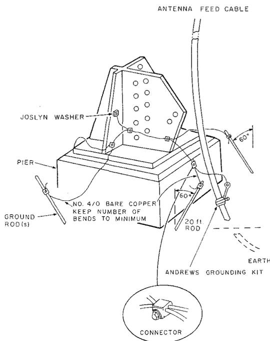
Fig. 1. Recommended ground connections at tower base.
