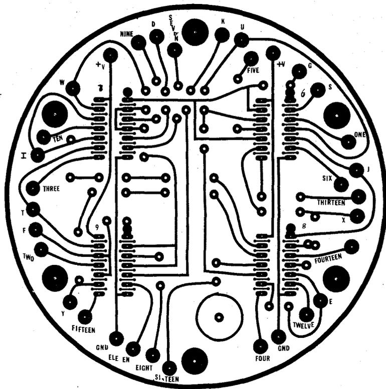
Fig. 11. Foil side of decoder board B.
