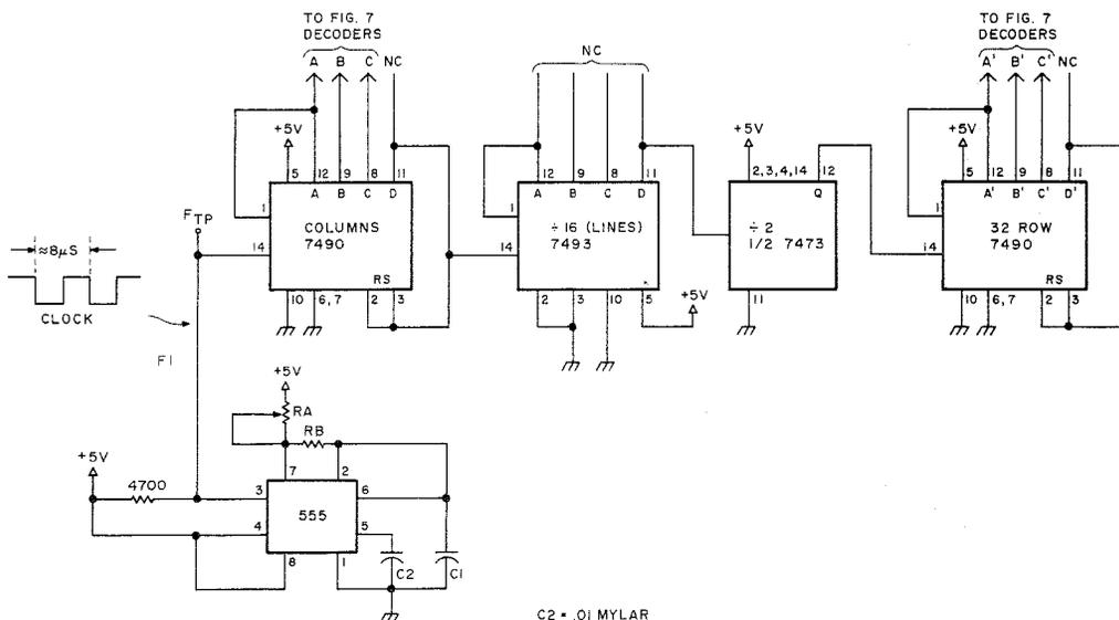
Fig. 3. Counter chain. Set for a frequency of 125 to 126 kHz at F<sub>TP</sub> test point. For this application, C<sub>1</sub> = 220 pF, R<sub>a</sub> = 10k thumbwheel PC pot, R<sub>b</sub> = 18k, 1/4-W fixed resistor. General formula is:  $f = 1/T = (1.44)/(R_a + 2R_b) \times C$ .
