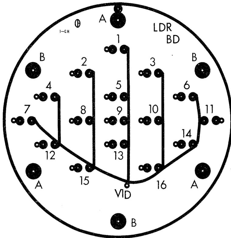
Fig. 2. Foil side of LDR board.
