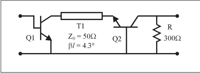
▲ **Figure 4. Resistive loading for improved stability.**
