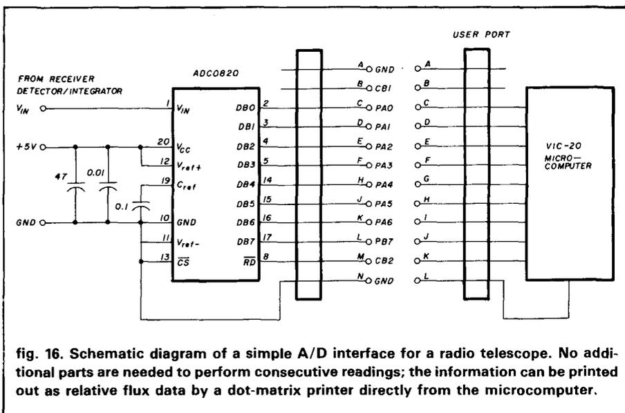
fig. 16. Schematic diagram of a simple A/D interface for a radio telescope. No additional parts are needed to perform consecutive readings; the information can be printed out as relative flux data by a dot-matrix printer directly from the microcomputer.
