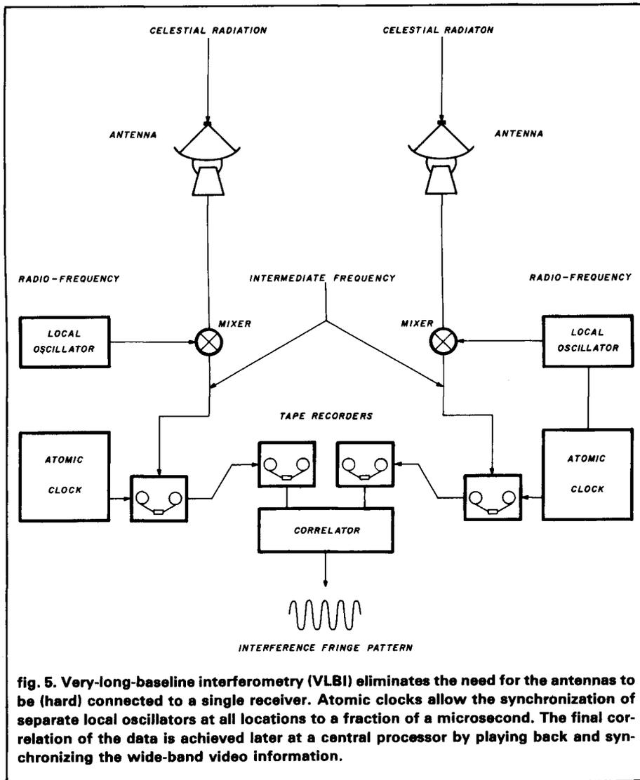
fig. 5. Very-long-baseline interferometry (VLBI) eliminates the need for the antennas to be (hard) connected to a single receiver. Atomic clocks allow the synchronization of separate local oscillators at all locations to a fraction of a microsecond. The final correlation of the data is achieved later at a central processor by playing back and synchronizing the wide-band video information.
