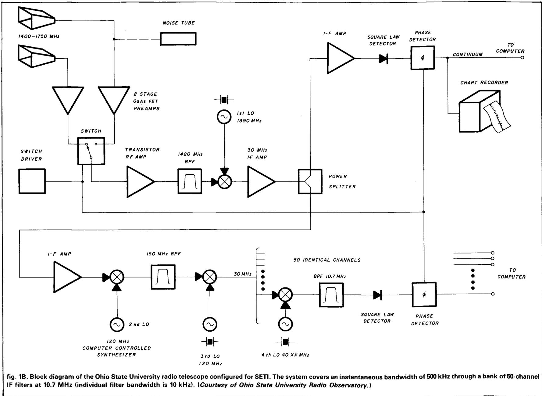
fig. 1B. Block diagram of the Ohio State University radio telescope configured for SETI. The system covers an instantaneous bandwidth of 500 kHz through a bank of 50-channel IF filters at 10.7 MHz (individual filter bandwidth is 10 kHz). (Courtesy of Ohio State University Radio Observatory.)
