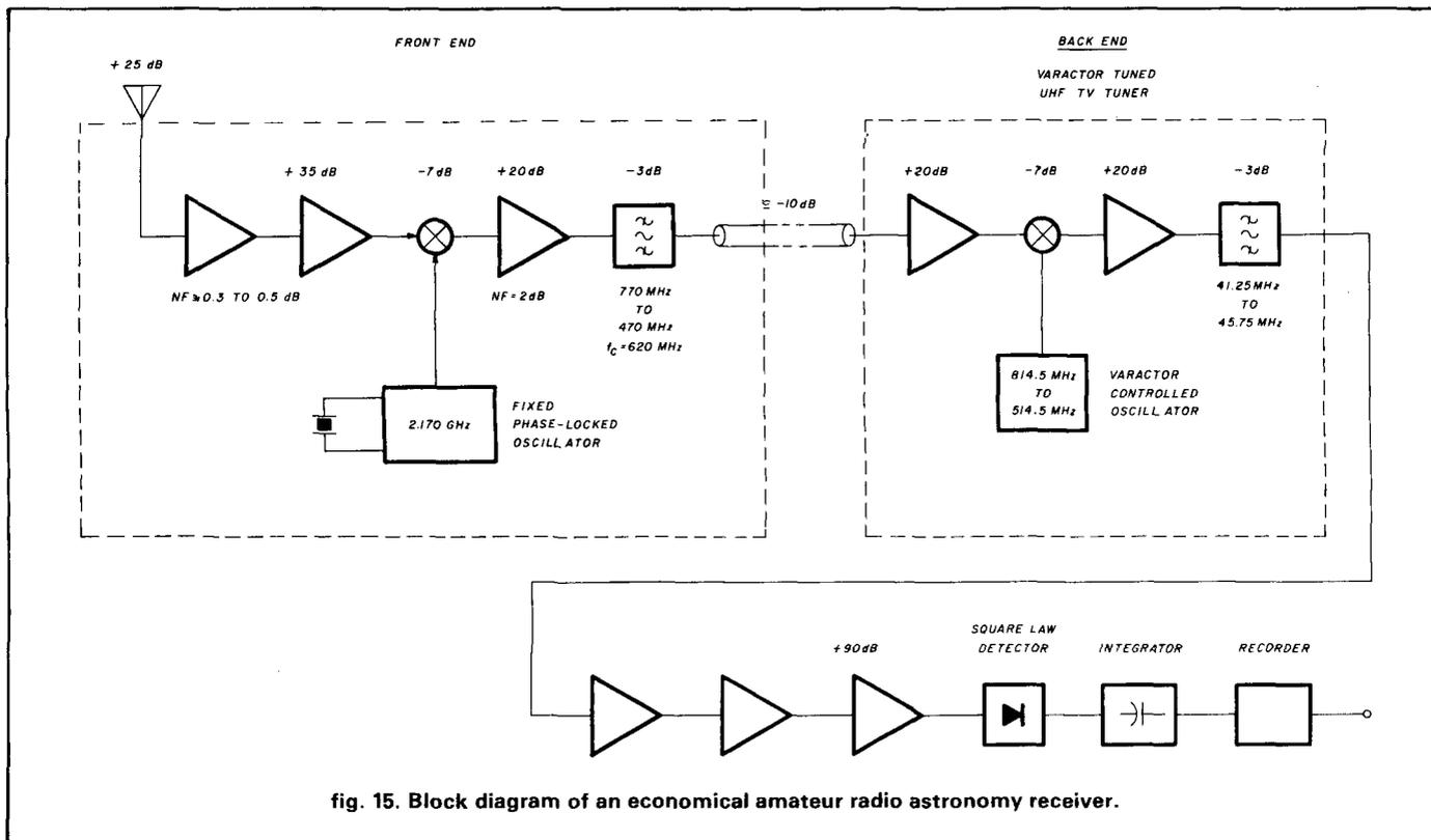
fig. 15. Block diagram of an economical amateur radio astronomy receiver.
