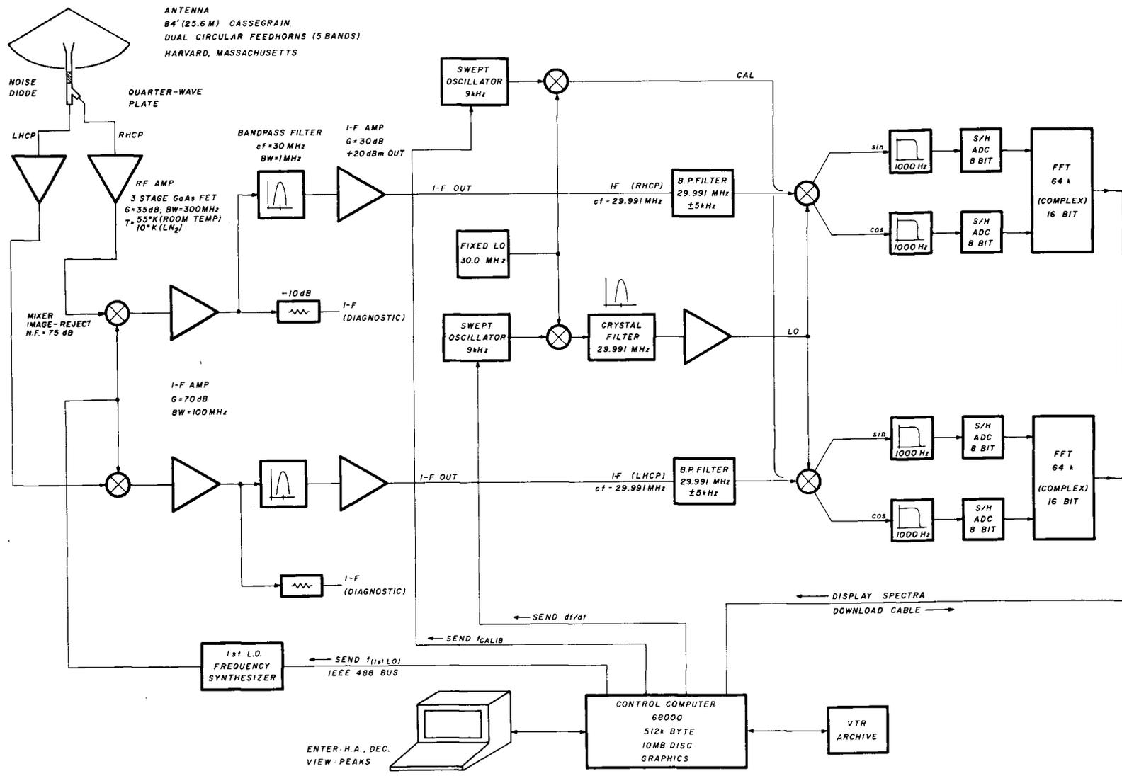
fig. 14. Block diagram of the Ultra-Narrowband SETI receiver used at Harvard University. The system uses an 84-foot (25.6 meter) equatorial radiotelescope with a single conversion dual polarization receiver intended for processing left and right circular polarizations at the same time. (Courtesy of Harvard University Physics Department.)
