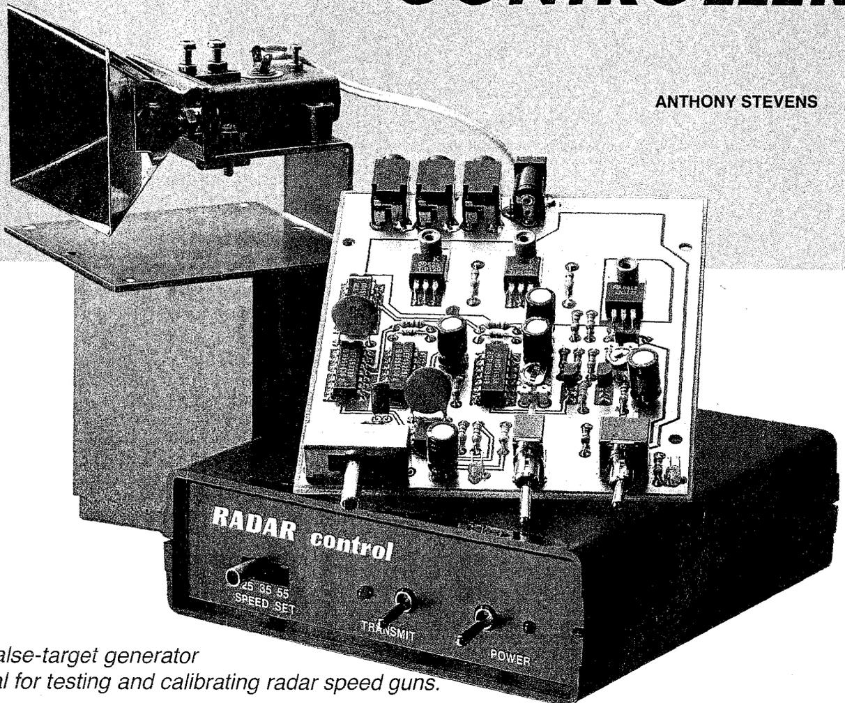
*This false-target generator is ideal for testing and calibrating radar speed guns.*
