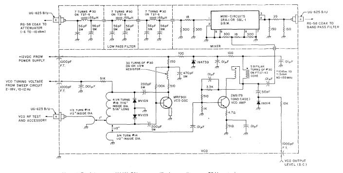
*Note 1.* Resistors are 1/4 W, 5%; unspecified capacitors are 50-V ceramic. *Note 2.* Capacitors marked "SM" are  $\pm$ 5% silver mica.
