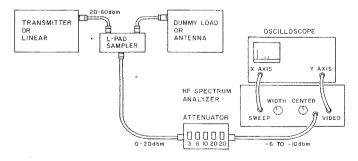
*Note 1.* Never hook transmitter or linear directly to step attenuator or analyzer. Always use L-pad sampler of the proper power rating. *Note 2.* Be sure transmitter, linear, L-pad, attenuator, analyzer, and scope are grounded.
