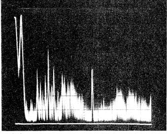
Photo L. 0-to-60-MHz spectrum on longwire antenna with my trusty but noisy computer on.
