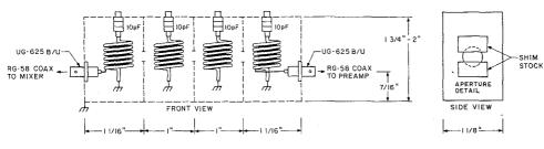
Note 1. Coils are 6 turns of #12, 1/2" inside diameter, 5/8" long, taps at 1/4 turn.
