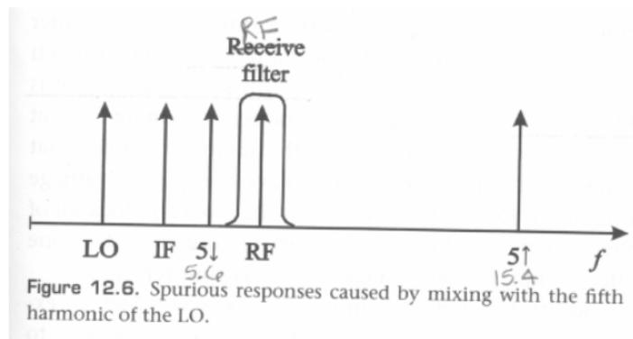
Of all the spurs, it turns out that  $f_{5\downarrow}$  is the one closest to the intended RF signal. It causes the **largest spurious response in the**
