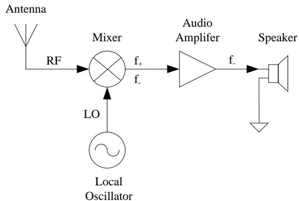
The frequencies internal to the direct conversion receiver are:
