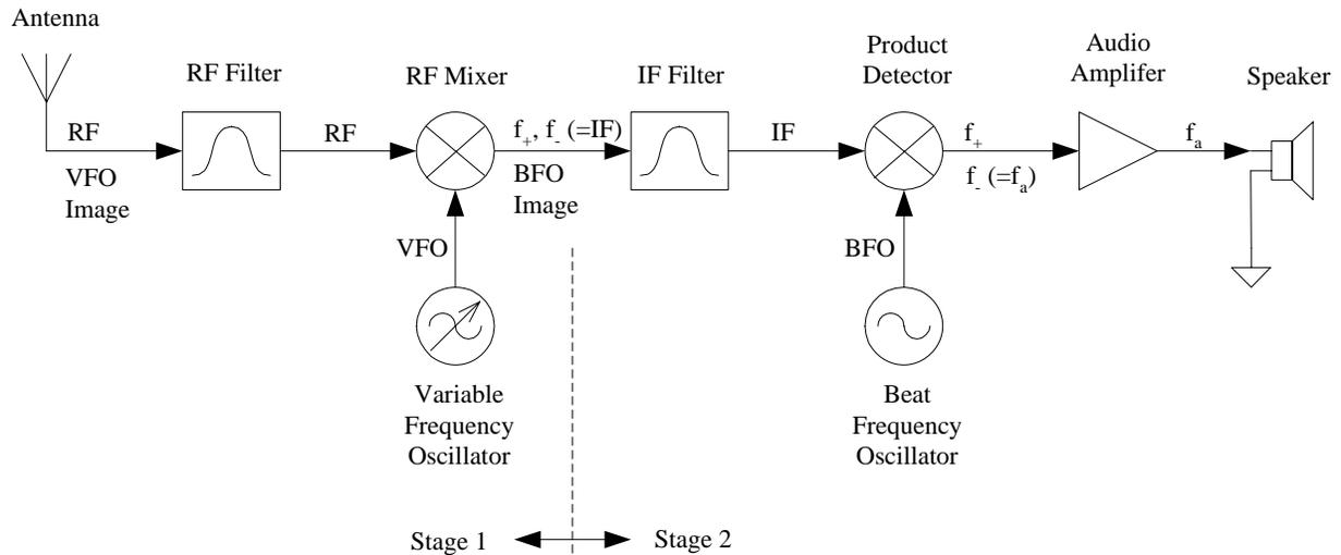
The frequencies internal to the superheterodyne receiver are:
