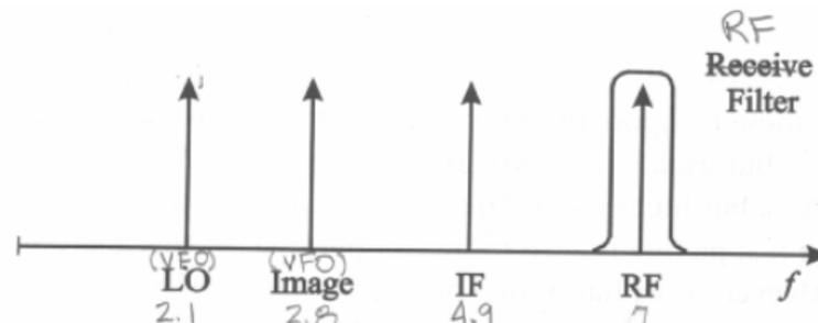
Figure 12.4. Mixer frequencies and the image frequency. A band-pass filter centered on the RF frequency prevents a signal at the image frequency from reaching the mixer.
