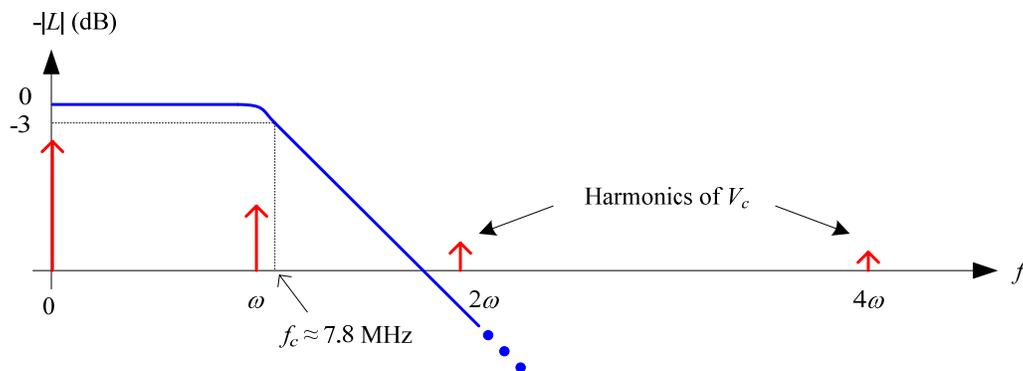
When the NorCal 40A is transmitting, the **Harmonic Filter** reduces the “higher-order harmonic” content in  $V_c$  (10.8) by significantly attenuating these frequency components.
