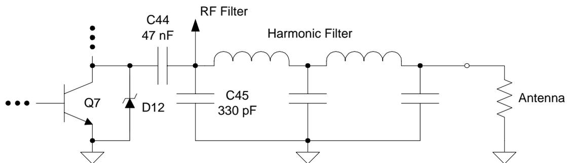
This capacitive discharge is due to **energy stored in C45 dissipating through Q7**. (Note that C44 is a dc blocking capacitor; hence, the voltage drop across C44 is very small, which implies the stored energy is also small.)
