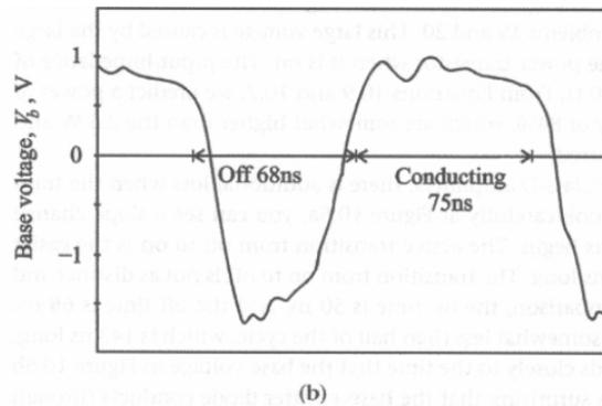
Figure 10.5. Voltages for the NorCal 40A Power Amplifier at 7 MHz. The output power is 2.5 W, with a supply voltage of 12.8 V and a supply current of 250 mA. The efficiency is 78%. Collector voltage (a), and base voltage (b).
