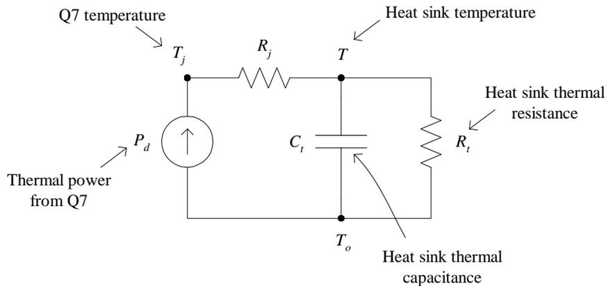
$R_j$  is the thermal resistance of the transistor-to-package interface. You often find this quantity specified by the manufacturer in the transistor datasheet.
