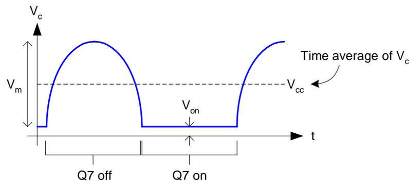
The transistor Q7 in the amplifier is either “off” (cutoff) or “on” (saturated). In-between these times, the transistor is active for a short time. (We’ll consider the active regions shortly.)
