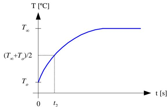
The behavior of this thermal circuit (and, consequently, the physical heat transfer phenomenon) is just like a single time constant **electrical circuit**. Very “cool”!
