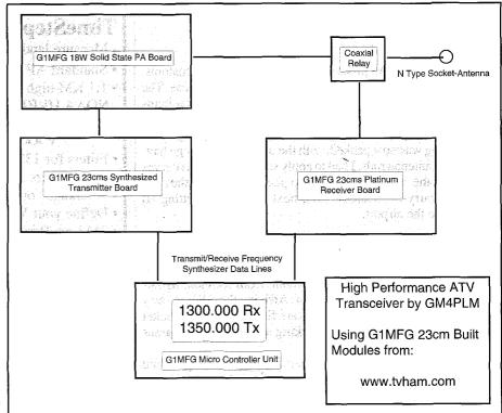
Figure 1. Block diagram of ATV station.
