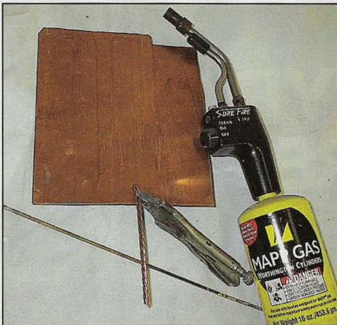
Ready to weld. A flat copper strap (scrap from a copper roof gutter installation that the author straightened out) with a stranded #6 copper ground wire. Locking-type pliers holding the wire in place, Silvaloy Excel 15 rod, and small handheld torch using MAPP gas are also shown.
