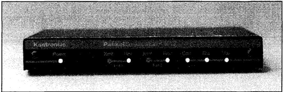
The KPC-9612 TNC is the centerpiece of Kantronics' packet paging system, with the latest release of the 9612 firmware supporting the mode. A personal computer may also be used to encode pager messages.
