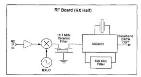
Figure 3. The receive portion of the WA4DSY modem design.
