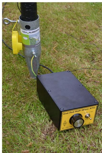
This suggested that a simple fixed tuning box (using a coax capacitor and set for around 21.650 MHz minimum SWR into 2000 Ohms) could give you a simple three-band vertical for 20, 17 and 15m.
