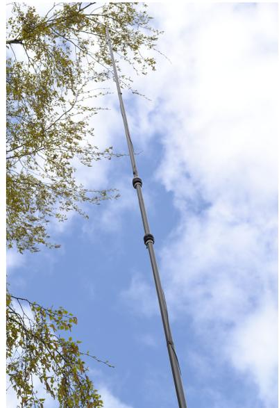
This actually makes sense as the end of an EFHW is at the same impedance as the end of a quarter-wave vertical, so a trap does the same thing. All you have to control is the resultant high feedpoint impedance. Doh! – why didn't I think of that earlier?
