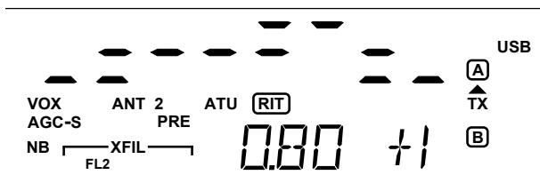
The center frequencies of the 8 audio EQ bands are 50, 100, 200, 400, 800, 1600, 2400, and 3200 Hz. To select a band to change, tap **0-7** on the keypad. For example, tapping **0** selects the 50-Hz band.
