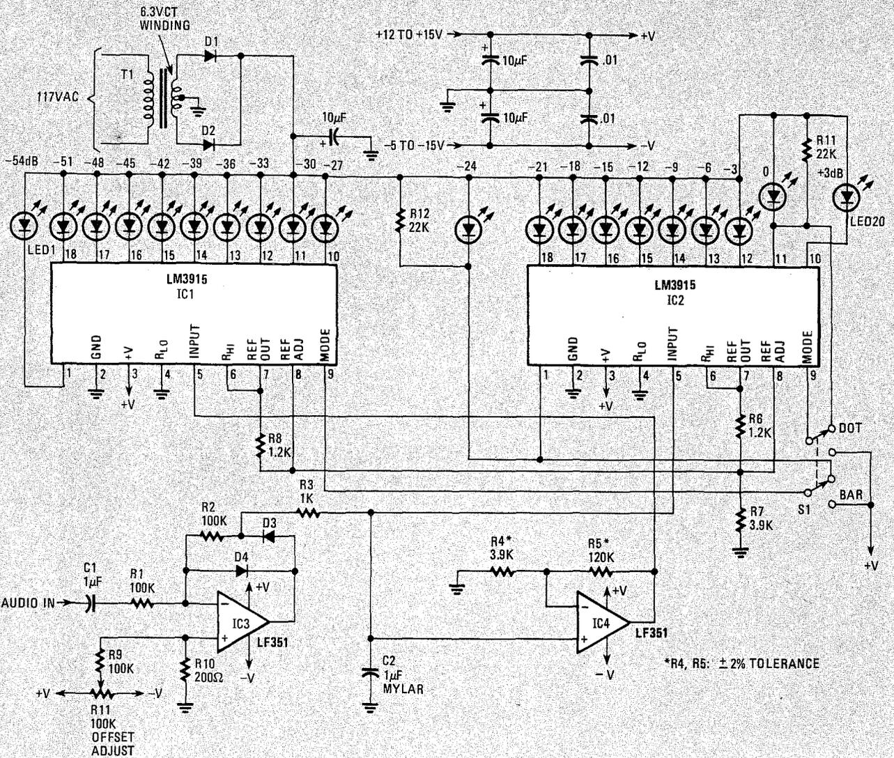
FIG. 6—TWO LM3915's can be cascaded together to obtain wide dynamic range. The circuit shown above is a peak-reading audio-level meter with a dynamic range of 60 dB.
