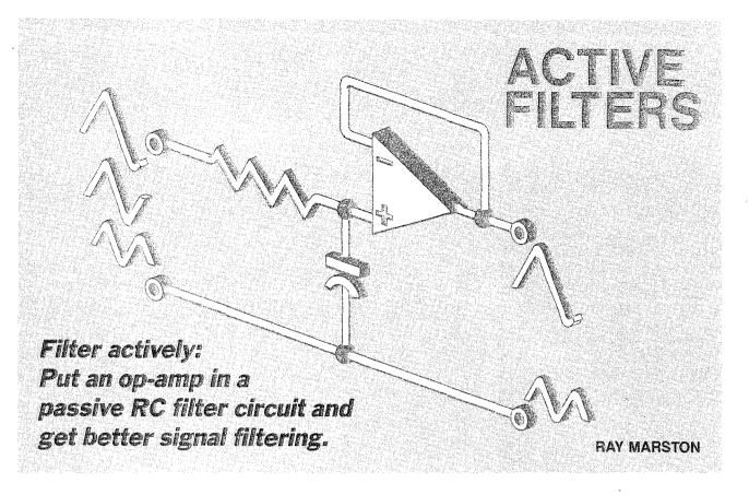
YOU CAN BOOST THE PERFORMANCE of any resistive-capacitive filter by combining it with one or more operational amplifiers. The result is an active filter that can do things passive filters can't do.
