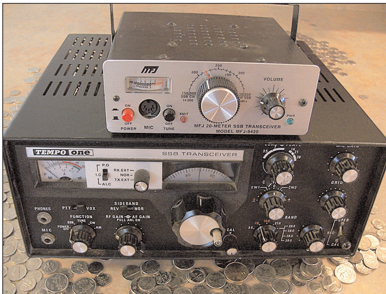
Photo B: Five bands and 100 watts vs. a single-band transceiver running 12 watts: It's a multiband Tempo One with a mono-band MFJ Enterprises MFJ-9420 transceiver sitting on top of it.
