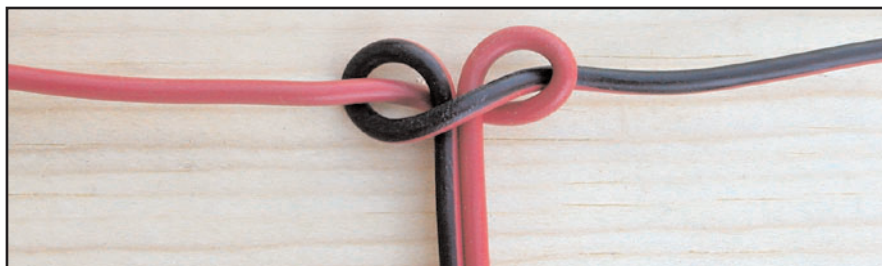
Figure 1: Jerry Hall, K1TD, in a 1979 QST article headlined “Zip Cord Antennas — Do They Work?” < http://bit.ly/ppGUdO > showed how to transition from feedline to antenna when using the same wire for both. This is an “electrician’s knot.” He explained that to tie the knot, first use the righthand conductor to form a loop, passing the wire behind the transmission line part and off to the left. Then pass the lefthand wire behind the left antenna wire, then in front of the transmission line part and through the loop already formed. Voila! ( Courtesy of K16SN )
