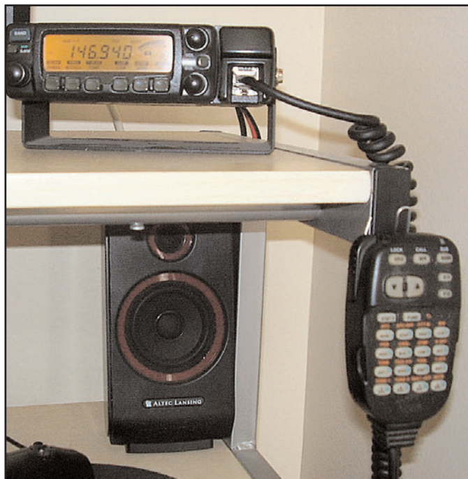
An ICOM 207H at VE6EFR is usually scanning between 146.94 and 147.06 MHz , as well as 147.495 MHz simplex.
