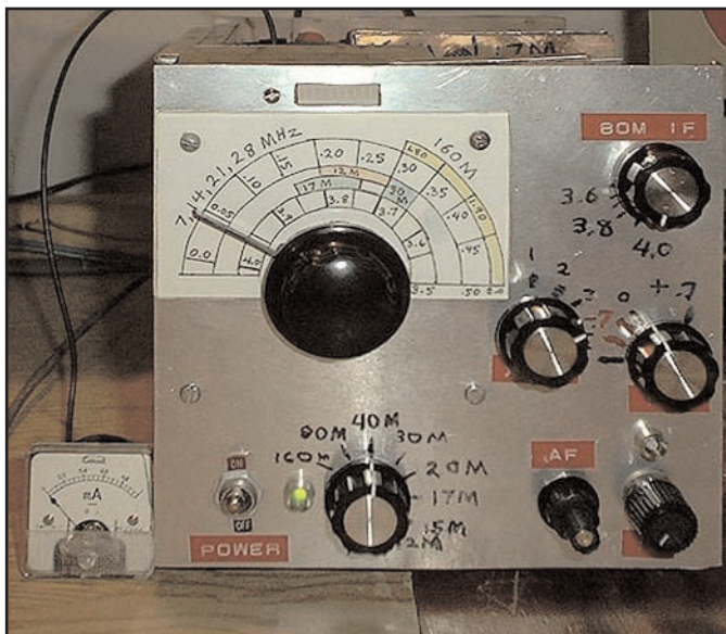
A hand-lettered front panel shows the coverage of KØIYE's multi-band receiver.
