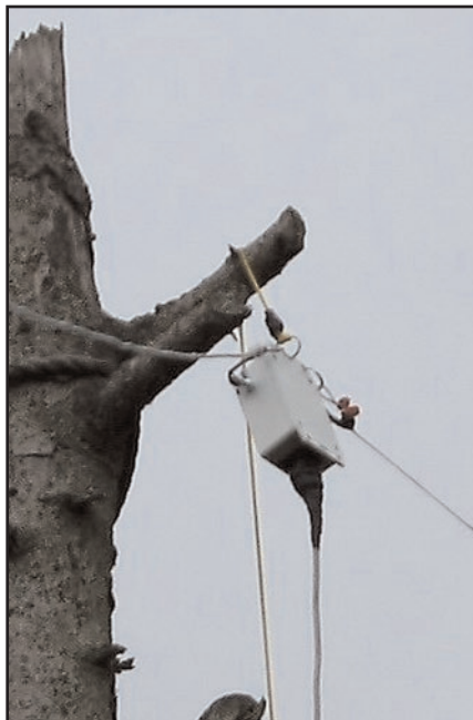
A balun is at the feed point of the Windom antenna used for amateur radio work at G4UCJ.
