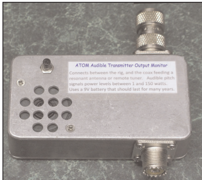
The “ATOM”, or Audible Transmitter Output Monitor, provides aural feedback that helps a blind user track power and tuning. (Photographs courtesy of K6KV)
