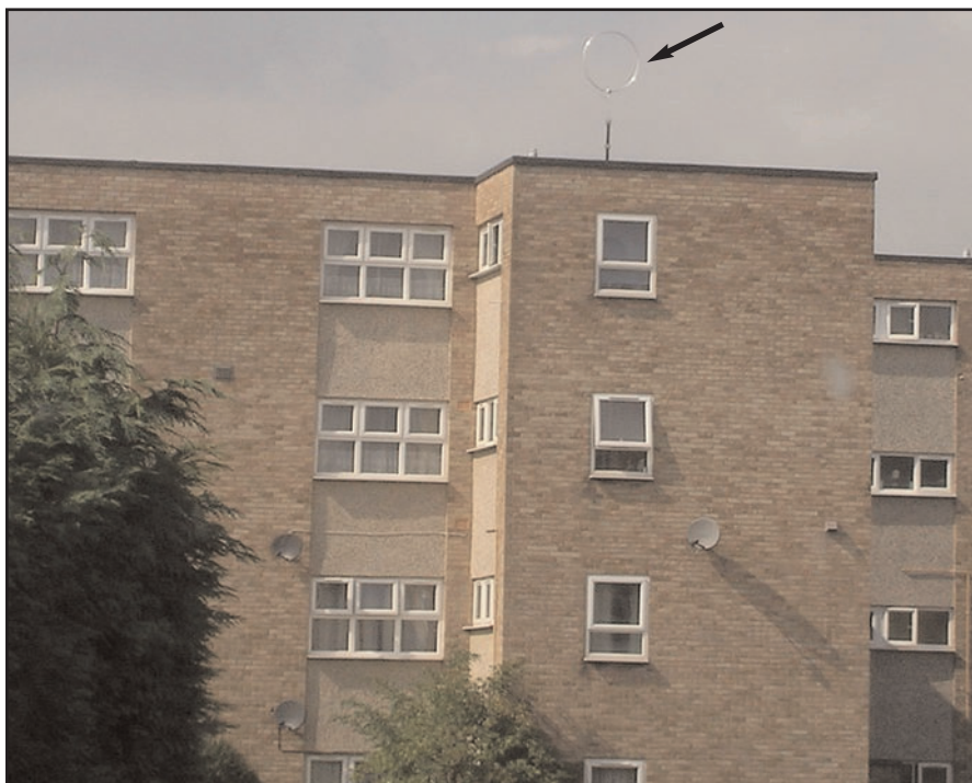
A photograph from G4UCJ's old QTH shows the Wellbrook receiving loop standing tall atop the multi-story building.
