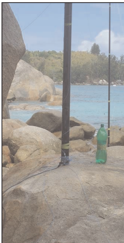
Here's the base of Battle Creek Special. The antenna was resonated for phone portion of 80-meters, but we used a Sprite Bottle Loading Coil to drag it down to the CW portion – with good results.
