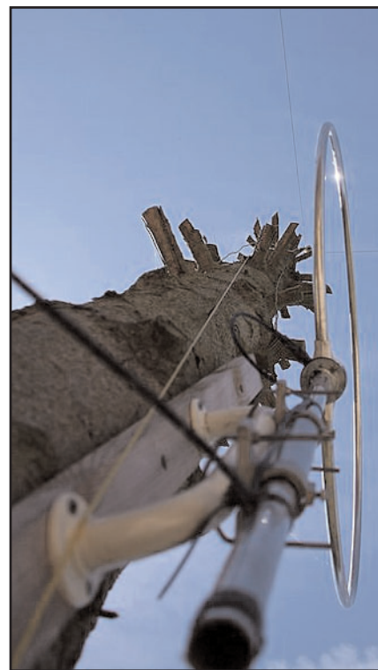
A Wellbrook active receiving loop antenna – one of G4UCJ’s keys to SWLing success – is attached to a tree below an off-center-fed dipole for 40 through 10 meters.
