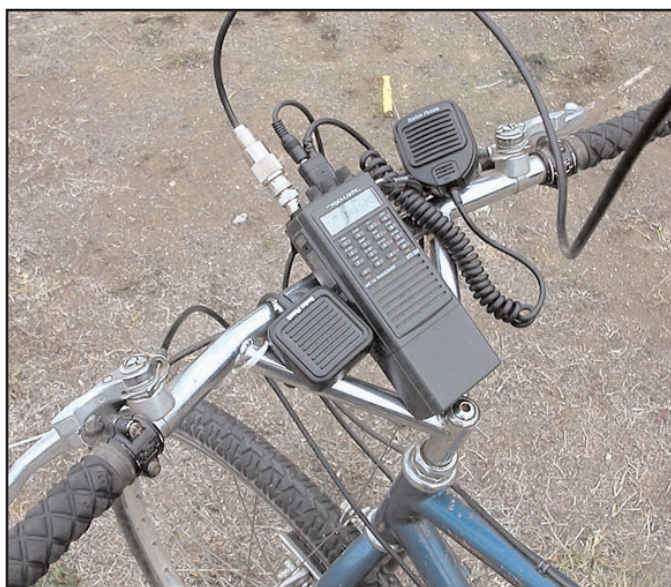
Handlebars secured with nylon strings make a nice surface on which to place the HTX-202, microphone and external speaker for 2-meter FM simplex and repeater operation.
