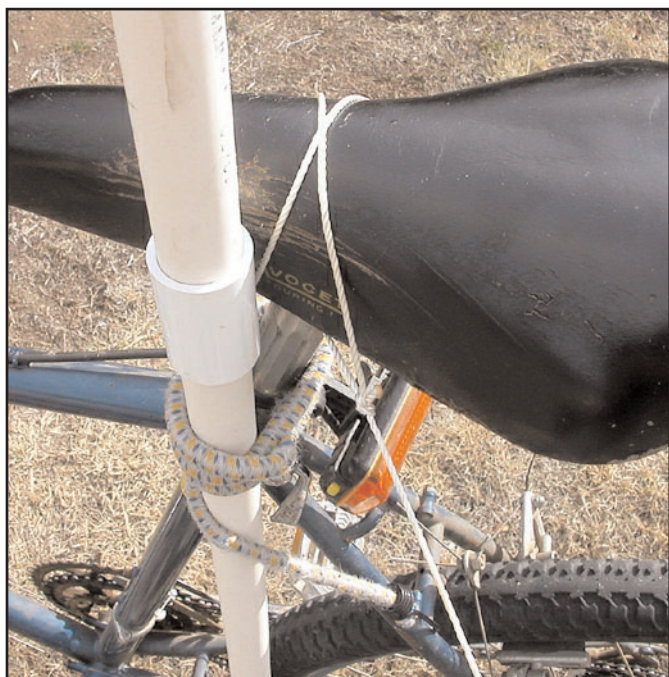
A three-foot-long bungee cord is used to strap the bottom part of the PVC mast to the bicycle frame.
