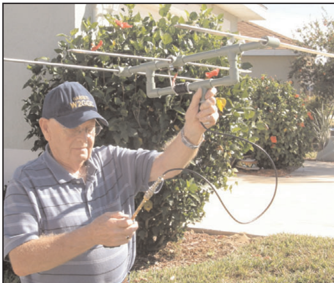
Garrett Collins, W2GGC, holds the 2-meter FM direction-finding 3-element beam built and used by the Royal Harbor Amateur Radio Club in its foxhunting activities.
