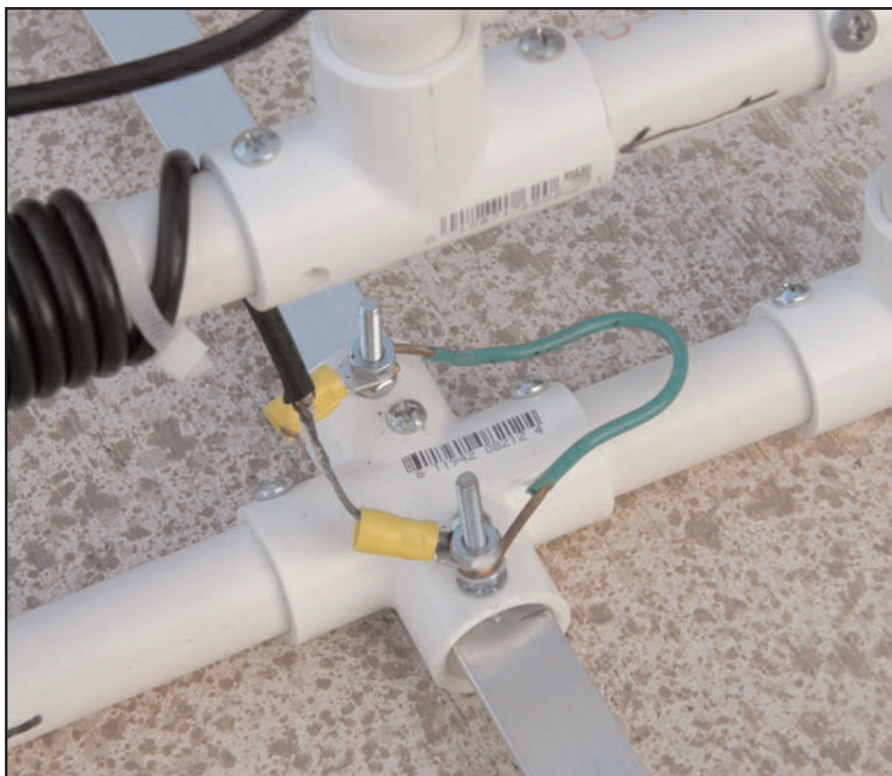
A close-up of the 2-meter beam's feed point shows the coiled balun, left, and the green hairpin impedance-matching system at the feed point used to get maximum efficiency from the antenna.
