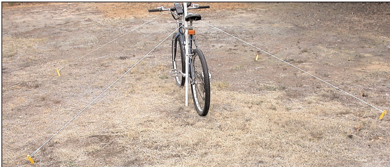
Four nylon strings and tent pegs make a feather-weight “kick stand” to keep your bike mast support upright, solid and secure.
