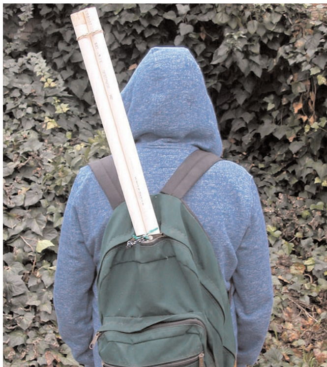
With the longest pieces just three feet in length, even a small backpack makes a nice carrying case for the portable mast. Fully loaded with antenna parts and radio gear, the sack weighs less than five pounds.
