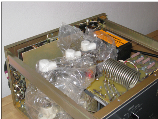
When shipping by sea container, precautions must be taken to ensure the equipment arrives in good shape. "There is actually a bigger story with this," NØVD said. PE2MC "started running the amp without realizing there was bubble wrap inside. Shortly afterward, the room was filled with the nasty aroma of melted plastic." (Courtesy of PE2MC)
