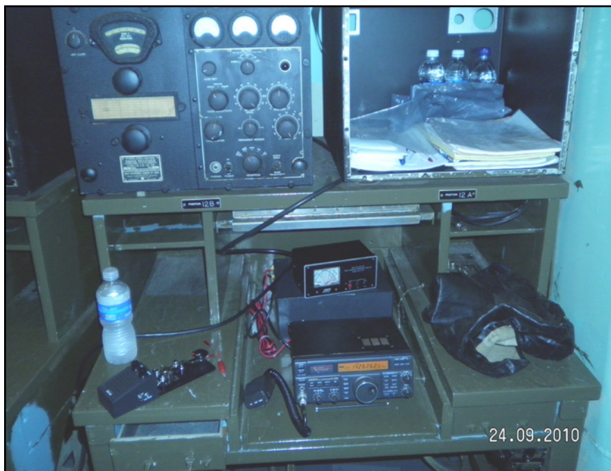
Aboard the ship, a vintage World War II receiver – at 82 lbs. – towers over a contemporary solid state transceiver, which tips the scales at about 8 lbs.
