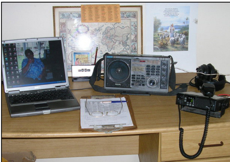
Next to ZS5DG's Phillips D2935 receiver is a Motorola GM 300 2-meter rig, connected to a 5/8-wave ground plane antenna for VHF operation
