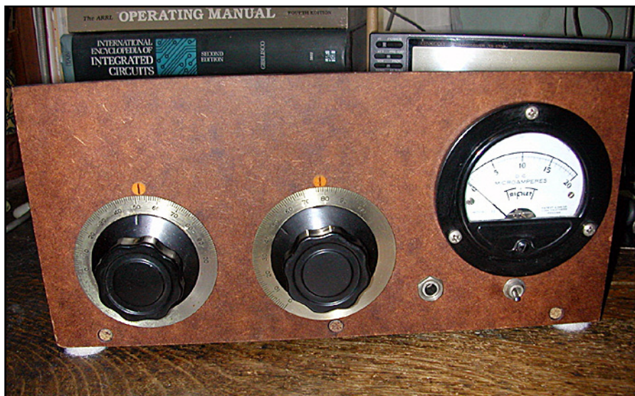
Two tuning capacitors and a 20 microampere meter dominate the front panel of the Myers Crystal Set receiver.
