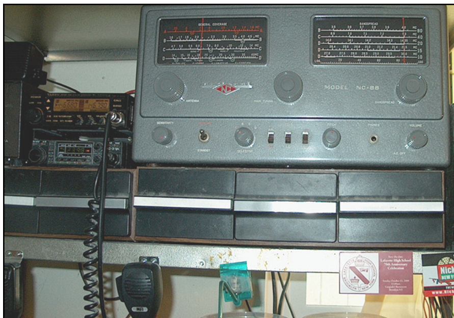
For the 2010 6 meter summer DX season, this National NC-88 receiver will be used with a converter designed and built in 1967 by WA6ITF using a 6BZ7 RF amplifier and a 6U8/6EA8 mixer.
