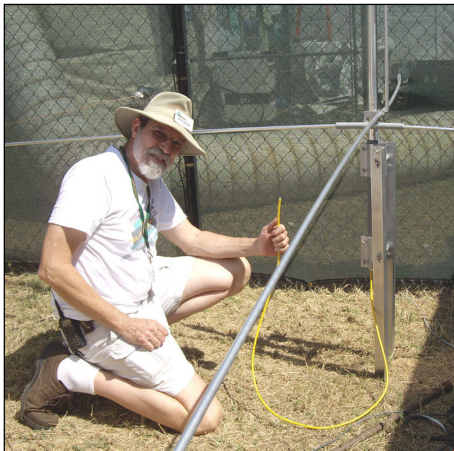
Bill Williams, AG4QX/NNNØYTD, Navy-Marine Corps MARS member from Tampa, discovers why SWR soared on the GAP Titan antenna used for HF transmission from the University of Miami Hospital's field installation: A cut counterpoise cable. (Courtesy of Gary Mentro N3OS/NNNØEKB.)
