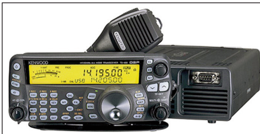
The Kenwood TS-480SAT, a popular radio with blind users, uses Morse audio prompts to indicate autotune status.
