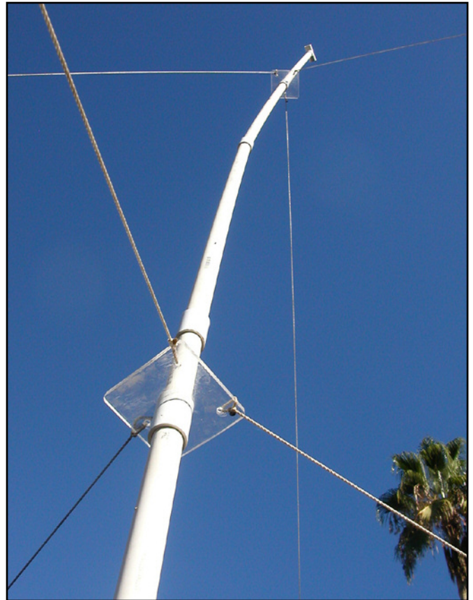
The KI6SN OM portable antenna mast is inexpensive, lightweight, easy to carry and a quick study in geometry to get in the air.
