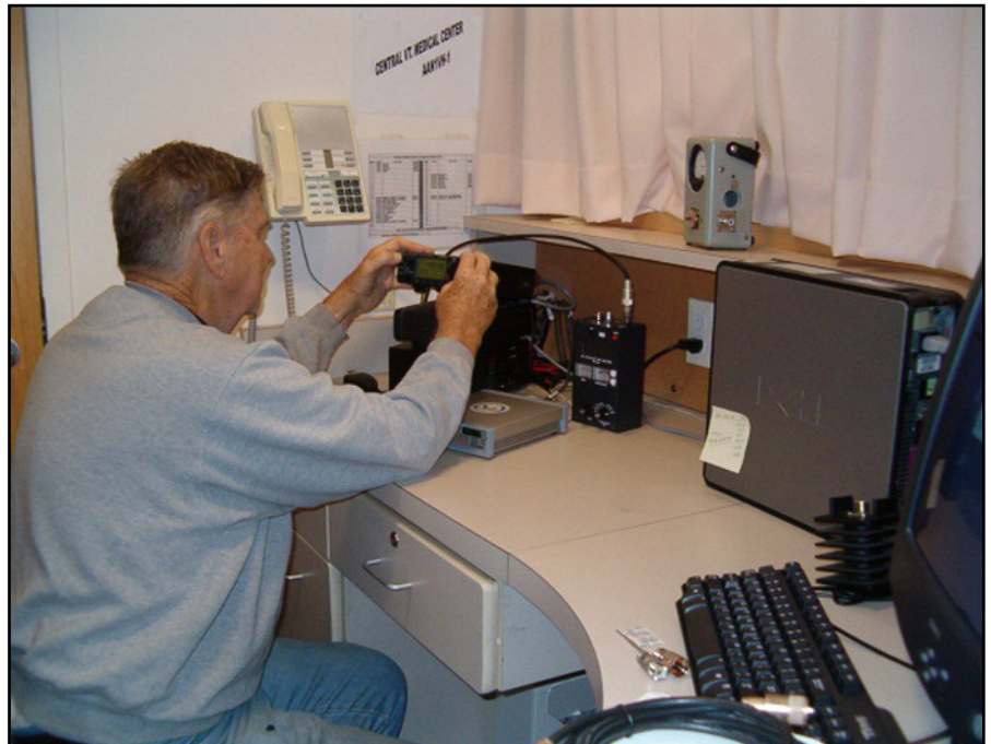
As Army MARS director for Northern New England, Ray Machel (KC1BT/AAA1NN) was an early champion of new technology. He's shown here installing the Winlink station at Central Vermont Medical Center, Barre, one of 67 Vermont agencies and offices he's set up for the MARS e-mail-over radio system. The state funded the IC-706 receivers, tuners and SCS pcIIpro Modems. (Photo: Betty Machel)
