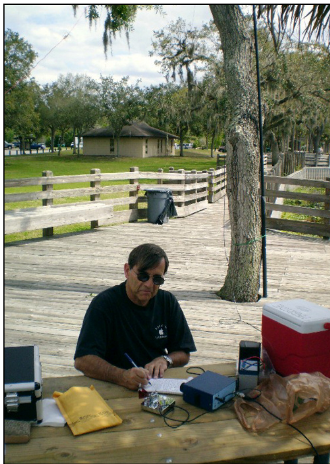
WA3ZBJ, with a set-up along the St. Johns River in DeLand FL, uses a Wilderness Radio Sierra transceiver portable with an inverted V antenna suspended from 33-foot pole shown in the background.
