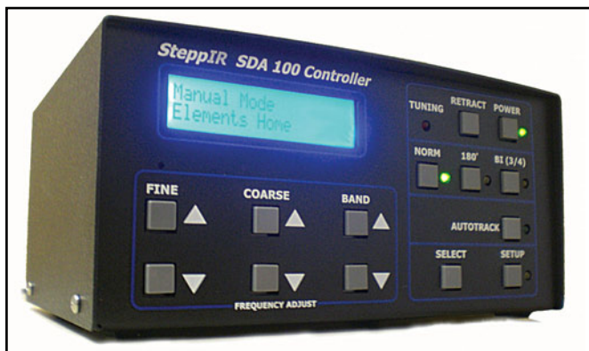
Photo A—SteppIR's new SDA-100 Controller has a larger LCD display than previous models, as well as dedicated LEDs for direction and antenna tuning, among other features.
