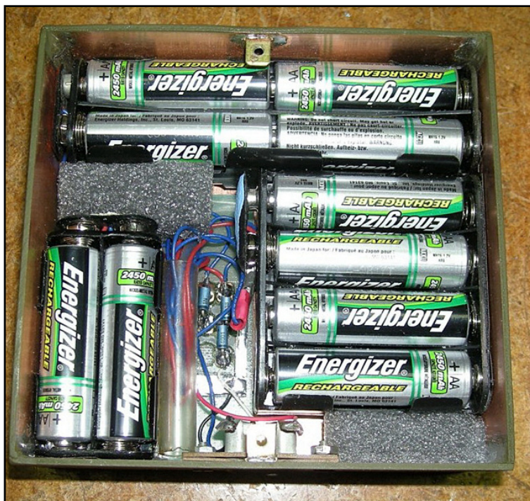
The PRC-64's voltage needs are provided by W6JRY in a specially-made field battery pack.
