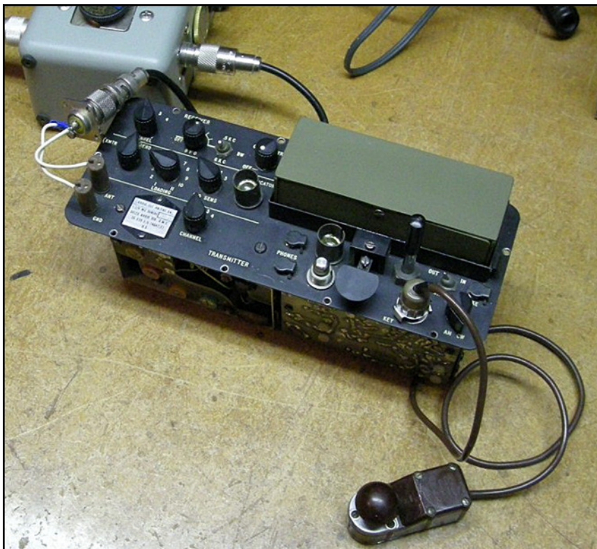
A recently restored PRC-64 Vietnam-era "spy radio" sits on the bench during testing at W6JRY.
