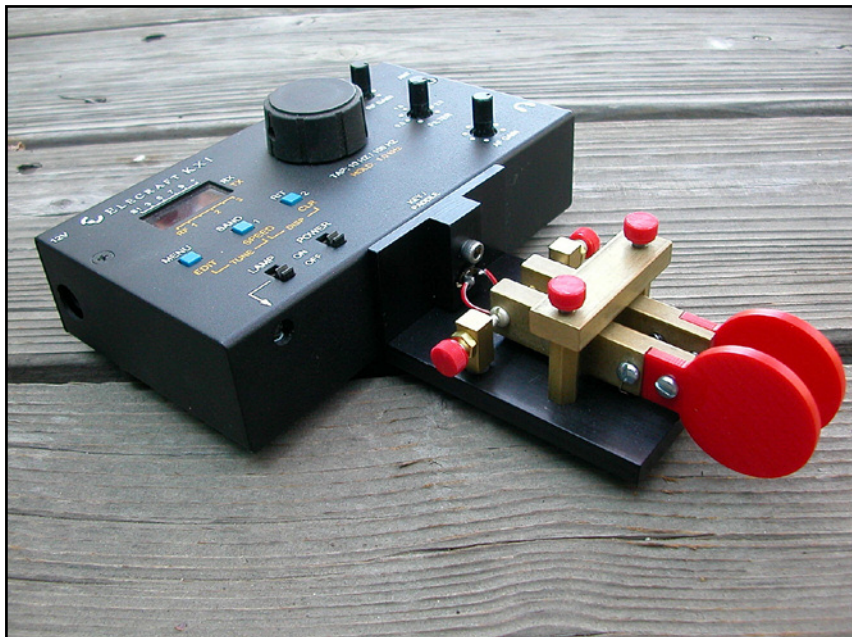
Docked to the Elecraft KX1 transceiver, the W5JH Baby Black Widow iambic keyer paddle is a perfect fit for operation in the field.
