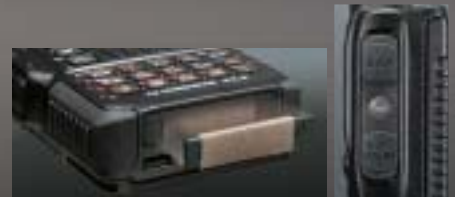
• Internal Bar Antenna (The photo is for illustrative purpose only)
