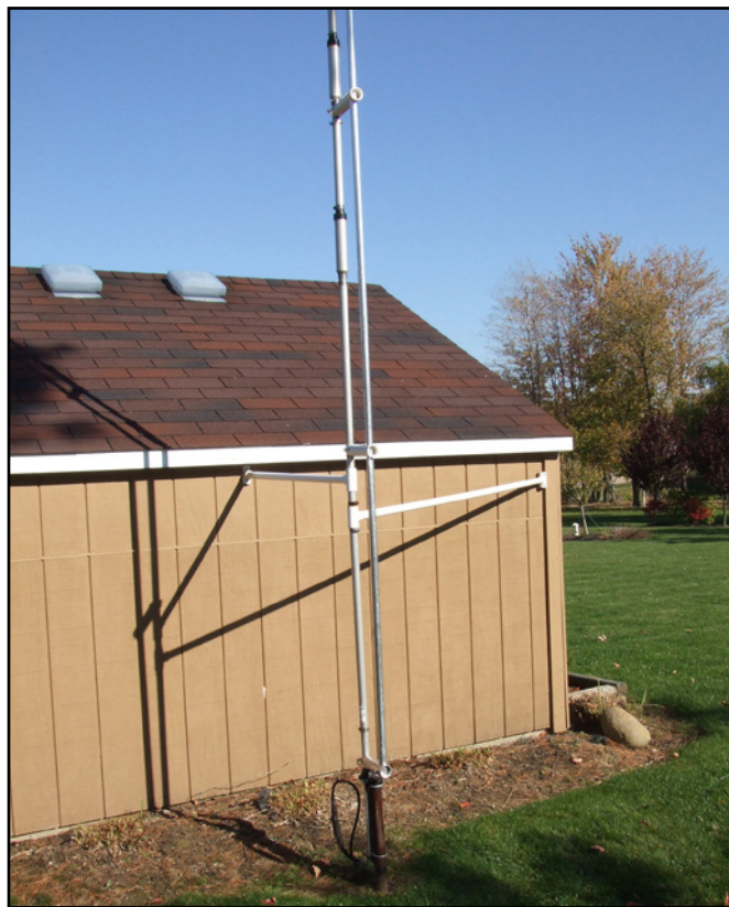
The finished 17-meter add-on attached to the Hustler antenna.
