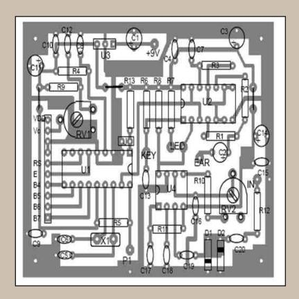
The whole circuit is mounted on a 60x80 mm PCB board. It is recommended to make use of small sized components (ceramic multilayers capacitors, low voltage electrolitics, ...) so as to make easier the assembling. The LCD display is connected by a 10 pole flat cable soldered to 2.54 mm standard connectors, as shown below
