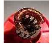
Solder each tap to each connection of your switch and stretch L1' (being 4 turns) at 1mm spacing and L1"(being only 3 turns) at 2 mm spacing. You can replace L1" by 3 turns of silver wire to allow better Q on higher frequencies (VHF).
