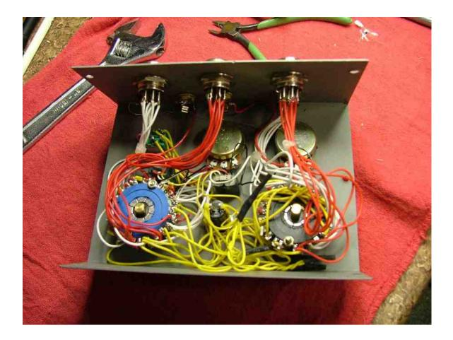
st I also installed a push button (push on – push off) switch that is also wired to pin 5 and 6 (ICOM push to talk pins). This allows keying while using headset or if keying is not done through the computer on the data mode.
