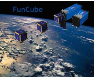
FUNcube will carry a UHF to VHF linear transponder that will have up to 1 watt and which can be used by Radio Amateurs worldwide for SSB and CW communications. Measuring just 10 \* 10 \* 10 cm, and with a mass of less than 1kg, it will be the smallest ever satellite to carry a linear transponder and the choice of frequencies will enable Radio Amateurs to use their existing VO-52 or DO-64 station.
