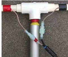
Fit a PL-259 on the other end of the coax(with appropriate reducers, depending on the size of the coax you are using). This completes the construction phase of the project.
