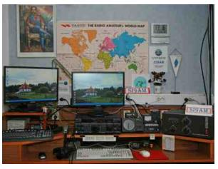
The station equipment consists of an FT 1000 MP with an ACOM 1000 amplifier. A 24-meter mast holds a tribander beam for 10/15/20 meters and a two-element for 40 meters. For other bands there are various wire antennas. A number of different software like TR, DX4WIN, HAM-Log, WIN-TEST and others is used for logging.
