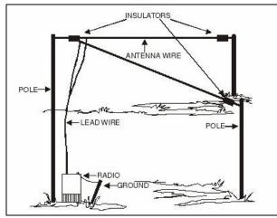
Fig. 1 Sloping vee antenna. The feedpoint should be about 40-50 feet high, and the end supports just a few feet high.
