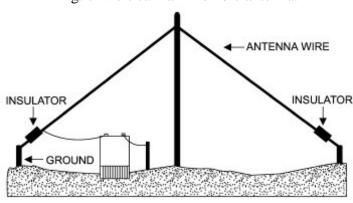
Fig. 7 Vertical half rhombic antenna.
