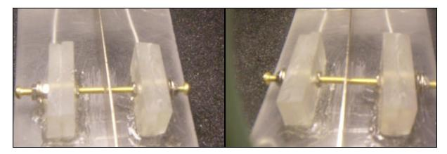
The Back Plate is shown here. Notice connecting wires from the Adjust Srews are run under the Base plate.
