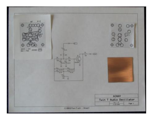
In this picture, I have the schematic of the project, the printed output from step 2 in the upper left corner of the schematic, the cropped printed output from step 3 in the upper right corner of the schematic and a 2" X 2" piece of PC board (Step 4) in the lower right corner of the schematic.
