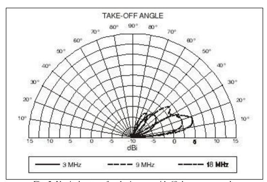
Fig. 5 Vertical pattern for sloping vee with 60 degree apex angle
