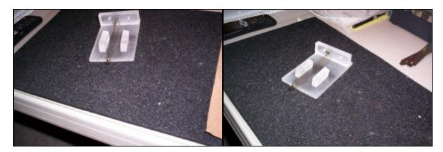
Here I've laid the arm in place to get an idea as to looks. After all of that I drilled from the bottom side some peggin' holes into which I epoxied in two 1/2" long 2-56 screws to reinforce the adjust screw plates. Most likely over kill but did it any way. You'll have to look close to see them.
