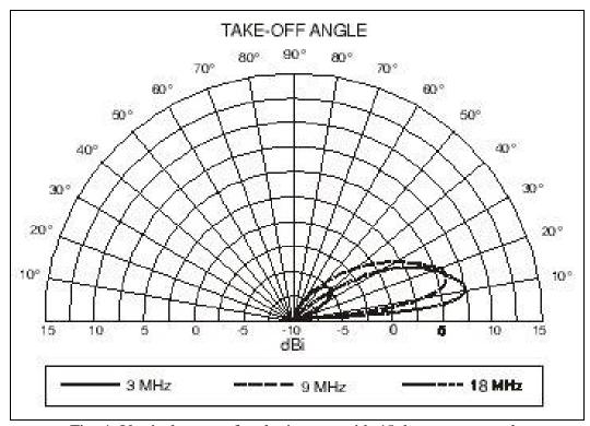
Fig. 4 Vertical pattern for sloping vee with 45 degree apex angle
