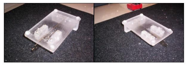
Here is the set up I used on the Adjustment Plates. The inside nut is epoxied on the Adjusting Plate. There 2 nuts and flat washers (6-32) to clamp the wires going to the Back Plate.
