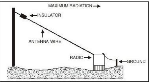
Fig. 6 Sloping wire antenna.
