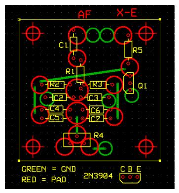
Dimensions are in real values. In other words, if I place a ¼" diameter circle on the drawing surface, it will be ¼" in diameter on the printed copy. A ¼ watt resistor is approximately 0.1" wide and approximately 0.4" long. On the printed copy, it will have those dimensions.
