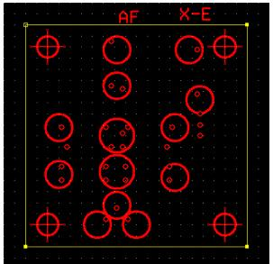
You will notice, right away, that all of the component outlines, ID's, and ground connections have disappeared. The very small circles are component connections for lead # 1 of the various components. For our purposes, ignore these. All that remains are the islands and the mounting hole circles. Cut the pattern along the board edges in the printout to produce the 2" X 2" cutting template.
