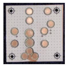
This is a picture of the PC board after all of the islands have been cut and the holes drilled for the mounting hardware. You will notice that the paper template is destroyed during the cutting process. The removed pieces of paper are caught in the bore of the cutting tools and should be removed.
