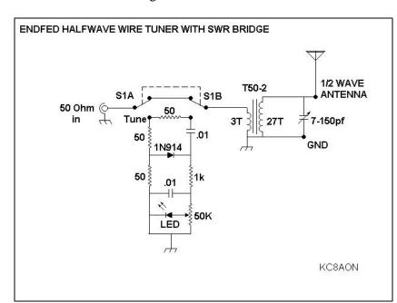
The 50 ohm side goes to the 3 turn link, and the hi Z antenna connects to the ungrounded end of the 27 turn winding. The variable capacitor connects across the antenna side from the ground to the antenna terminal. The variable capacitor in this tiny tuner was salvaged from an old AM broadcast band transistor radio that I picked up at a flea market for 50 cents! If you see these old radios cheap at flea markets, grab them - the vari caps are valuable!
