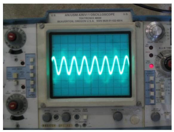
This is a picture of the sine wave output from our project board. The vertical scale is 5mv/division and the horizontal scale is 1 ms/division. As displayed, the output is 12.5mv PP at approximately is 714 Hz (5 complete cycles in 7 ms).
