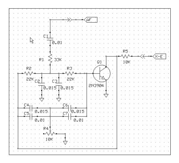
I allowed ExpressSCH to automatically assign component ID's. Take note of the "double arrows". This is a custom component that I built and use to indicate external connections to a project board. The connections with arrows pointing inward (towards board components) are inputs. Likewise, those pointing away from board components are outputs.
