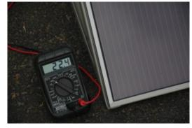
Shown here is the no-load output voltage (on the small DDM) in an almost clear sky. As you can I extend my "RF Ecology" idea to include natural power see, the no-load voltage is around 22VDC. This drops to about 14-15 volts under load
