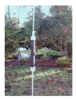
Above, you will see the components of the PAC-12, 2 threaded 12" rods, couplers, feed point (BNC connector on aluminum flat bar to which radials are attached), 72" telescoping whip with coupler, and two coils, 40m and 17m. In the swamp I use a 24" base section to push down into the sand. The second picture captures the 40m coil in action in my backyard with the swamp in the background.
