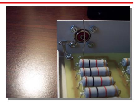
Once I had it all finished, I hooked up the Ohm Meter and checked my work. The display bounces between 50 and 51 Ohms as shown in the photo. On another Ohm meter it's exactly 50 Ohms, which is what Ohm's Law says it ought to be.
