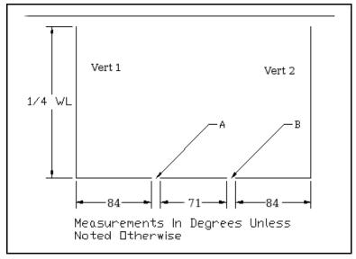
84 degrees at 7050 will be 90 degrees at 7553 kHz (7050 X 90/84). The 71 degree phase line will be 90 degrees at 8936 kHz (7050 x 90/71).
