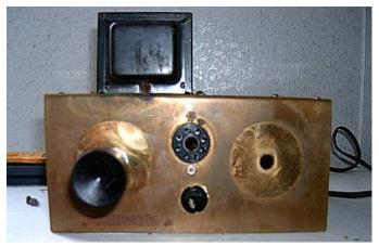
Power cord from a defunct soldering gun brings line voltage in to S1, then to F1 (4 amp glass fuse), then to T1. Output of T1 to the bridge rectifier goes through the filter caps R1 and R2. The voltage after the rectifier was 180vdc. After calculating that I needed 1800 ohms of resistance to my regulator tube, I used two 1000 ohm 1/2w resistors in series. The regulated voltage then goes to the octal socket pins 1&8 with 2&3 being the filament voltage.
