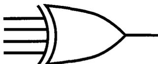
*Figure 7-7 - alternative representation of 4-bit parity calculator*
