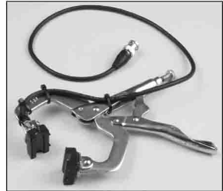
Figure A—A handy probe is made by attaching the two halves of a modified ferrite core to a Vise Grip clamp. Plastic ties secure the cable to the clamp.
