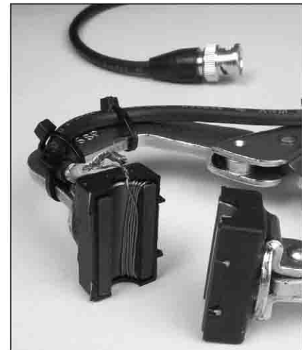
Figure B—Close up view of the modified ferrite core wound with a few turns of enameled wire.
