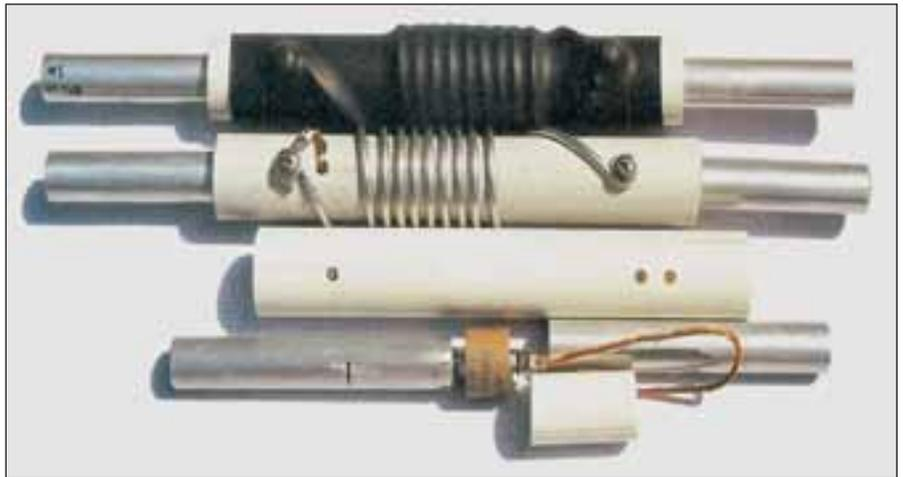
**Figure 2—**The trap assembly is shown in various stages of fabrication. The mechanical components are detailed in the drawing package available on the ARRLWeb site. This photo shows the 50 pF NPO capacitor attached to its trap terminal, complete with a flexible wire. The coil form and insert are also shown. Although this particular design used a shrink-sleeve cover, the final design used two coats of gray epoxy instead.
