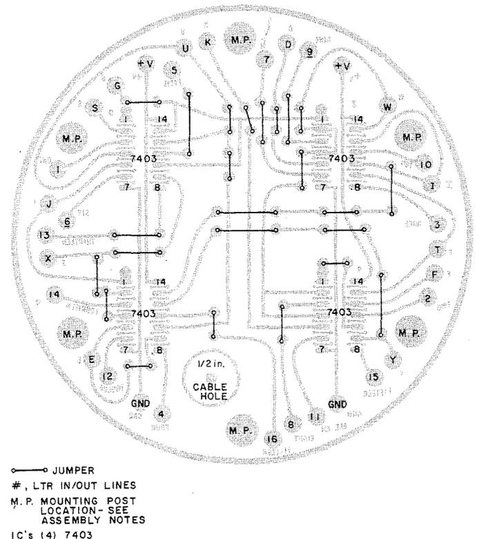
Fig. 12. Component side of decoder board B. Numbers and letters indicate proper placement of input/output leads to other boards. Solid lines connecting dots are jumper leads on component side.
