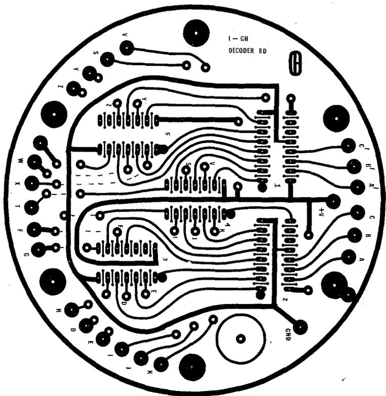
Fig. 8. Foil side of decoder board A.
