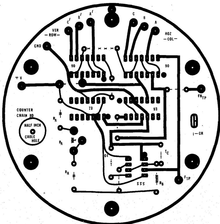
Fig. 5. Foil side of counter chain board.
